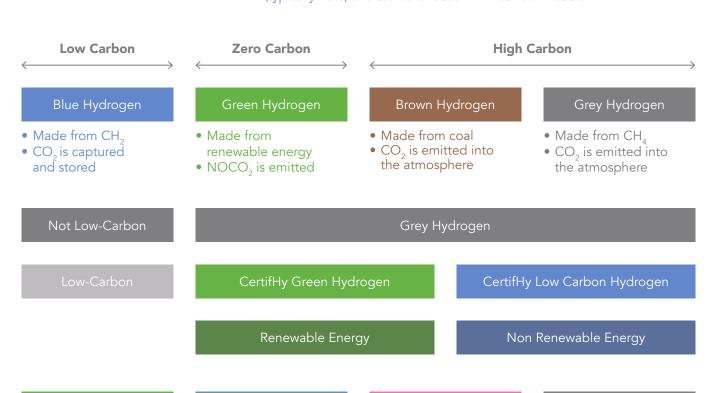
Hydrogen produced by electrolysis of water, using electricity from renewable sources like hydropower, wind, and solar. Zero carbon emissions are produced.
